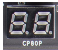
Debug LED with CPU Temperature Monitor
