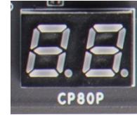
Debug LED with CPU Temperature Monitor
