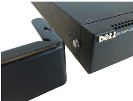
Figure 1-6. Fixation des supports
