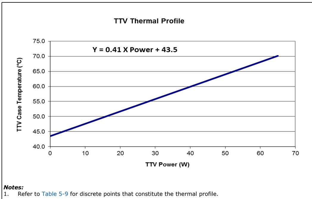
**Table 5-9. Thermal Test Vehicle Thermal Profile for PCG 2015A Processor (Sheet 1 of 2)**
