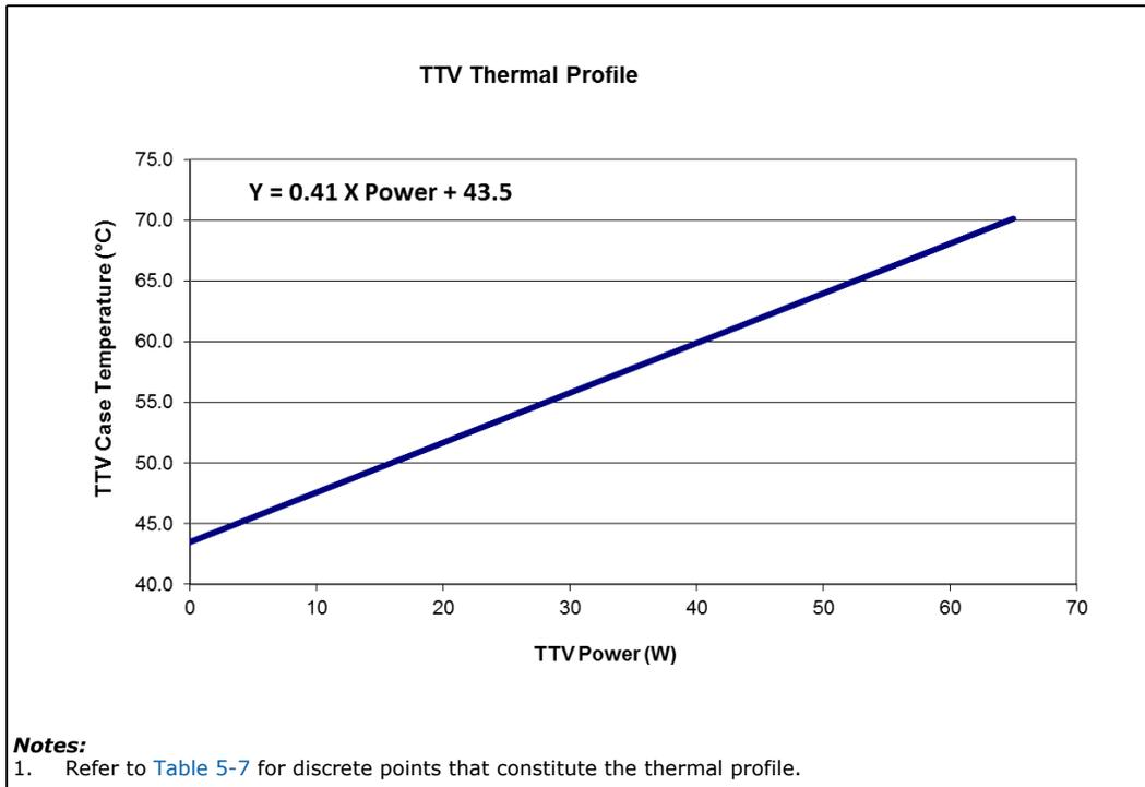
**Table 5-7. Thermal Test Vehicle Thermal Profile for PCG 2015C Processor (Sheet 1 of 2)**
