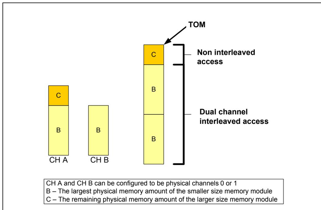
**Dual-Channel Symmetric Mode (Interleaved Mode)**
