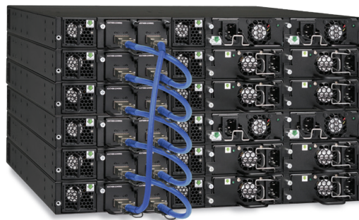
Figure 1: Up to 12 Ruckus ICX 7450 switches can be stacked together using two full-duplex QSFP+ 40 Gbps ports that provide a fully redundant backplane with 960 Gbps of stacking bandwidth.
